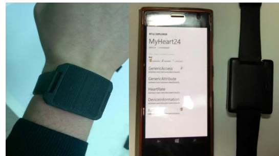
Fig. 2: The device for diagnosing the CVS status, which is connected to the Microsoft Lumia 730 smartphone via the Bluetooth protocol and transmits the data to the doctor's workplace (the smartphone is running a BTLE Explorer application designed to analyze devices developed using the Bluetooth Smart services and features)
