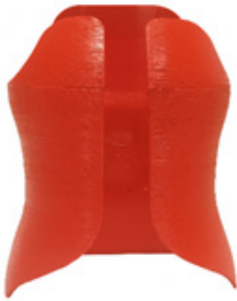
Fig. 4. 3D scoliotic brace fabricated using 3D printing technology
