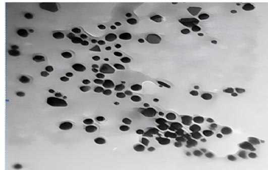
**Fig. 3.** SEM image of gold nanoparticles
