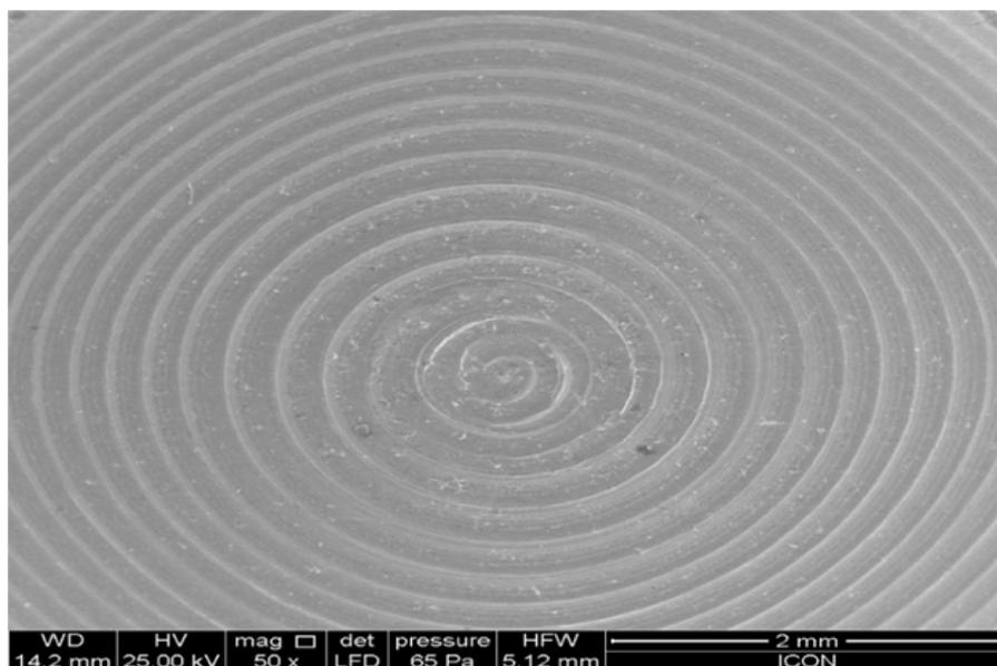
**Fig. 1.** SEM image of the uncoated commercially pure titanium disc
