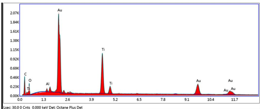
**Fig. 4.** EDAX of surface-treated titanium disc
