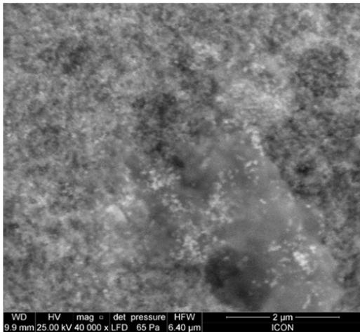
**Fig. 2.** SEM image of gold nanoparticles coated titanium disc surfaces
