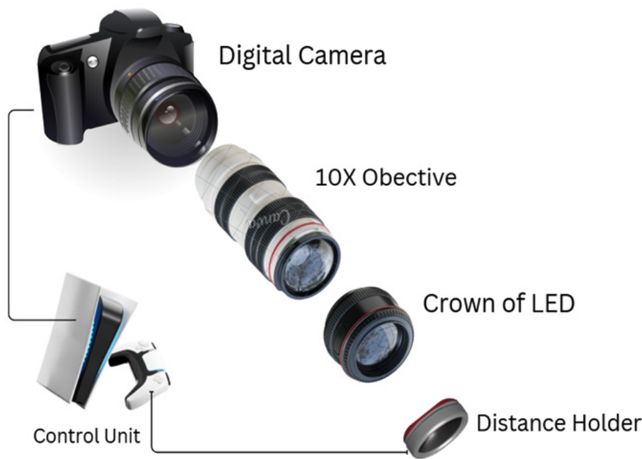
Fig. 1. Basic structure of a Dermatoscope
