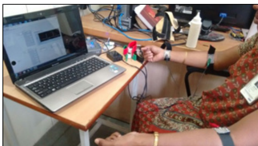
Fig. 6. Experiment Setup with Textile Electrodes
