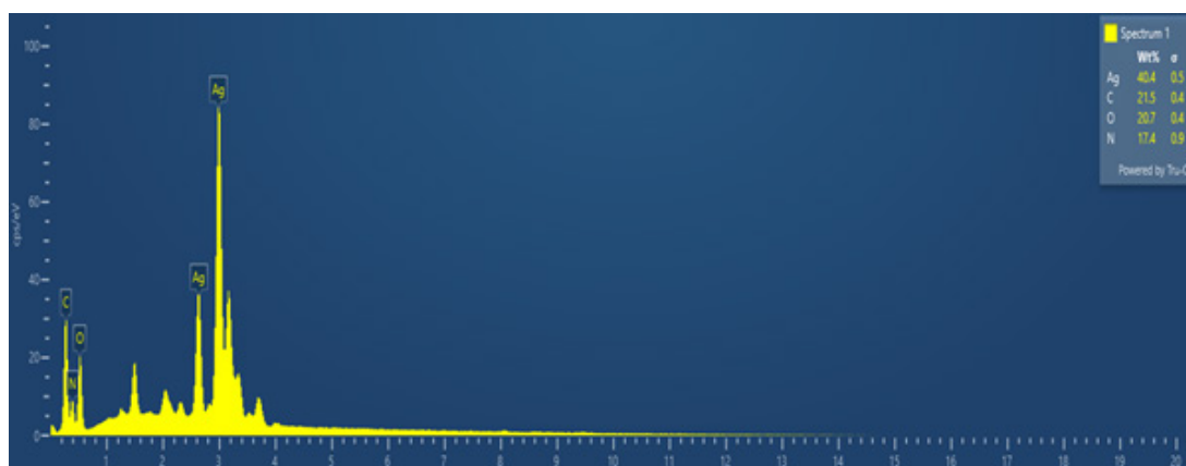
Fig. 4. Energy dispersive X ray analysis of MO - silver nanoparticles mouthwash demonstrated 40% of silver and 60% of MO
