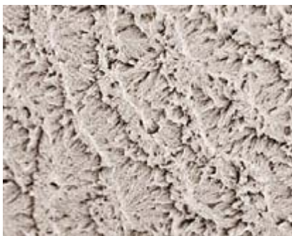
Enamel after 37 % phosphoric acid etching
