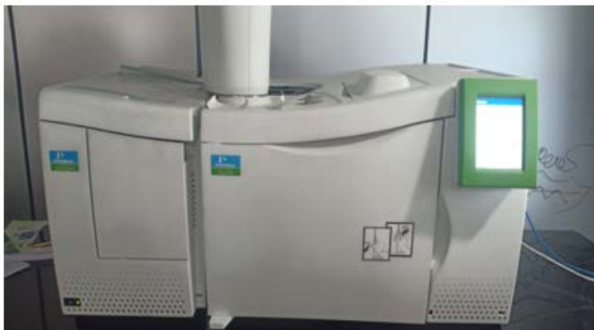
Fig. 4. The model (PerkinElmer Clarus 680) GC-MS was used for chromatographic analysis
