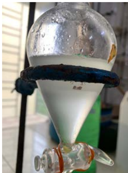
Fig. 2. Nifedipine dissolved in upper layer of 1-octanol and lower layer of distilled water
