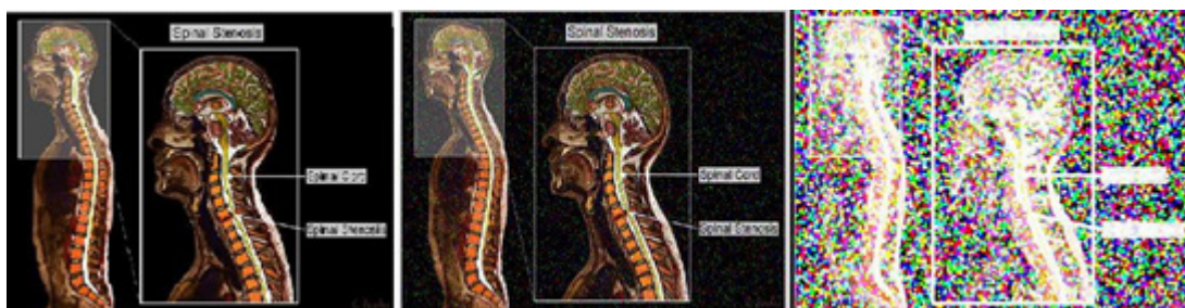
Fig. 9. (i) Input Image (ii) Salt & Pepper crashed Image (iii) Image clarified with MAX5x5 filter masks
