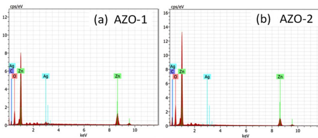
**Fig. 3.** EDX images for ZnO/Ag nanoparticles synthesized by (a) single step procedure (AZO-1) and (b) double step procedure (AZO-2)
