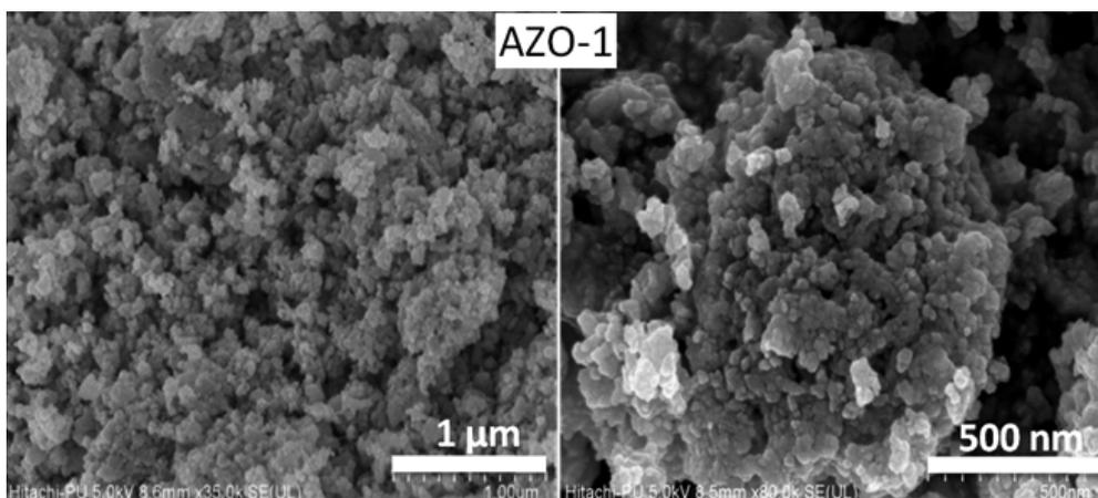
**Fig. 2(a).** FE-SEM images for ZnO/Ag nanoparticles (AZO-1) synthesized by single step procedure at the scale of 1  $\mu$ m and 500 nm
