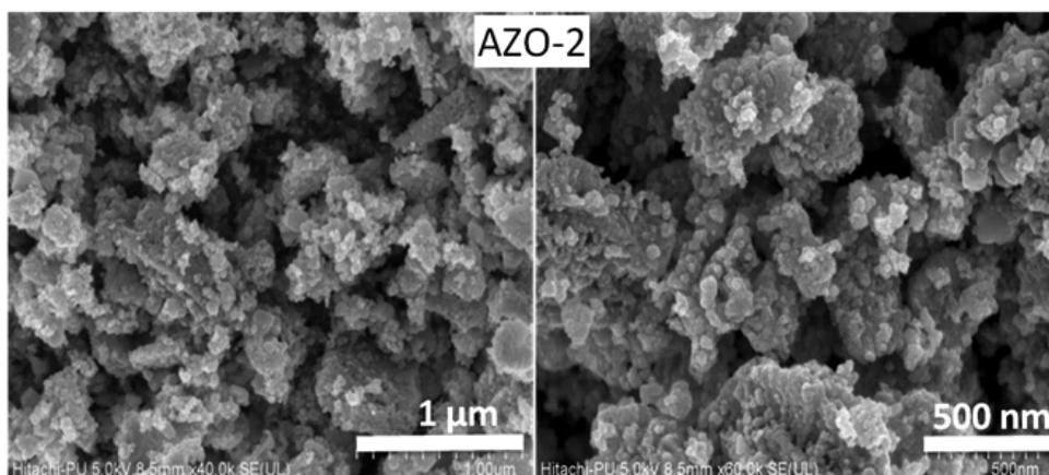
**Fig. 2(b).** FE-SEM images for ZnO/Ag nanoparticles (AZO-2) synthesized by double step procedure at the scale of 1  $\mu$ m and 500 nm
