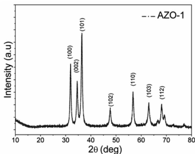
Fig. 1(a). XRD spectra for ZnO/Ag nanoparticles (AZO-1) synthesized by single step procedure
