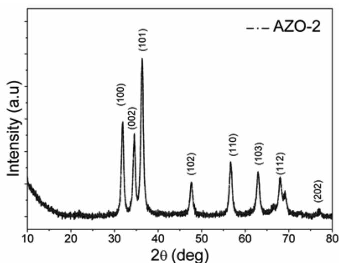
Fig. 1(b). XRD spectra for ZnO/Ag nanoparticles (AZO-2) synthesized by double step procedure
