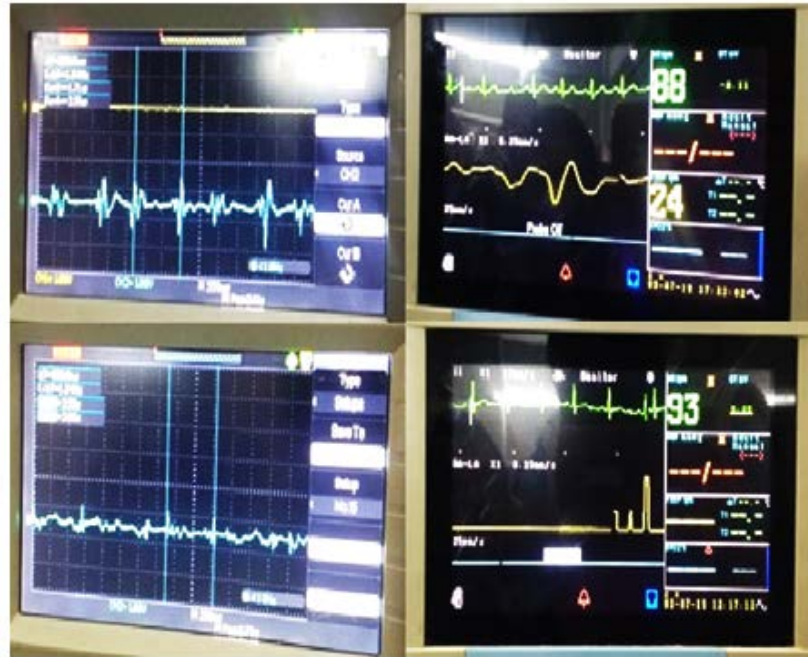
Fig. 7. Recordings of Non-Contact Method and its comparison with that of Patient Monitor
