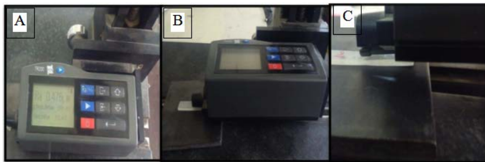
Fig. 6. Surface roughness testing. A: Profilometer; B& C: specimen testing at different points
