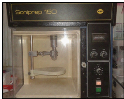
Fig. 1: Probe sonication apparatus
