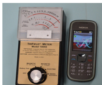
Fig.1. a) A 30-egg incubator with a mobile placed inside b) TriField Meter showing high electromagnetic while receiving a call
