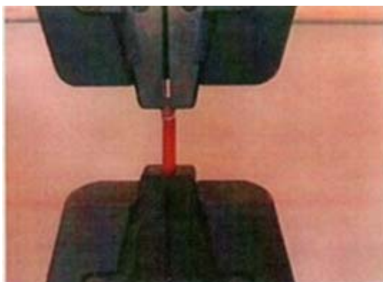
Fig. 7: specimen after fracture on instron machine
