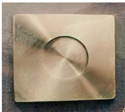
Fig. 1: Stainless steel die for making samples for contact angle measurement
