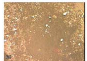
Fig. 8: Microphotograph Showing SM Bhasma etched with Ferric chloride (400X)
