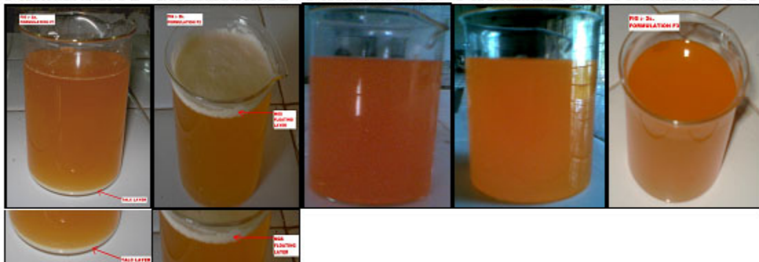
Fig. 3: Compatibility studies of different lubricants
