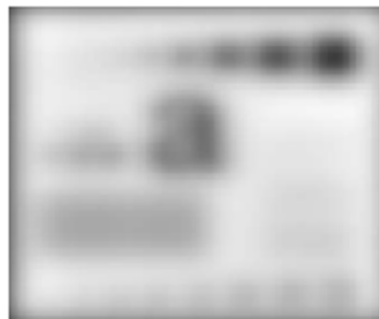
Fig. 11: result of filtering with Cutoff frequency set at radius value 10
