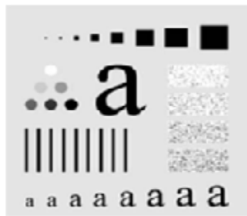
Fig. 14: result of filtering with Cutoff frequency set at radius value 160
