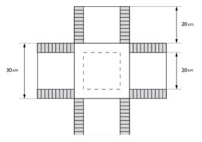
The coil is made of several single coils with air-gap between them for the possibility of airing. (Fig.4).
