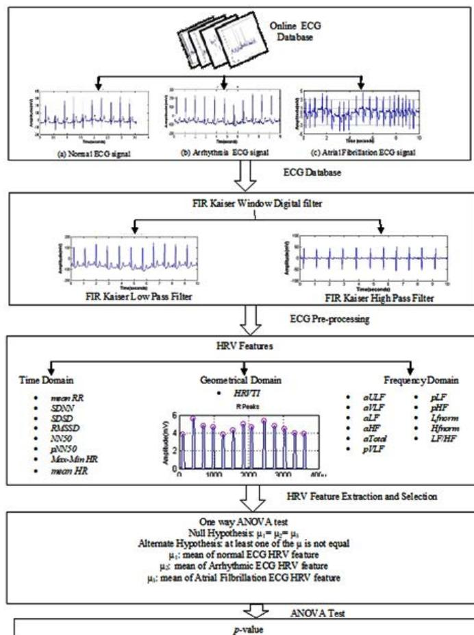
Fig. 1. Block diagram of methodology of HRV Feature processing
