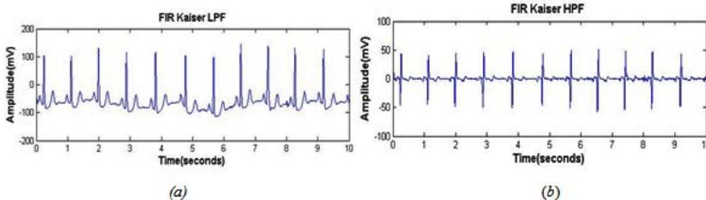
Fig. 4. Filtered ECG signal using FIR Kaiser Window (a) LPF for PLI removal (b) HPF for BLW removal
