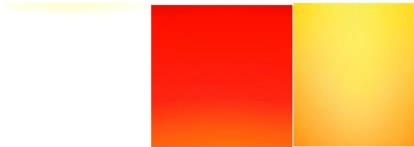
Fig. 7.1. Bad Capture-1 [Chatterjee et al.] Frame with average pixel intensity > 250 – 254 on red channel:
