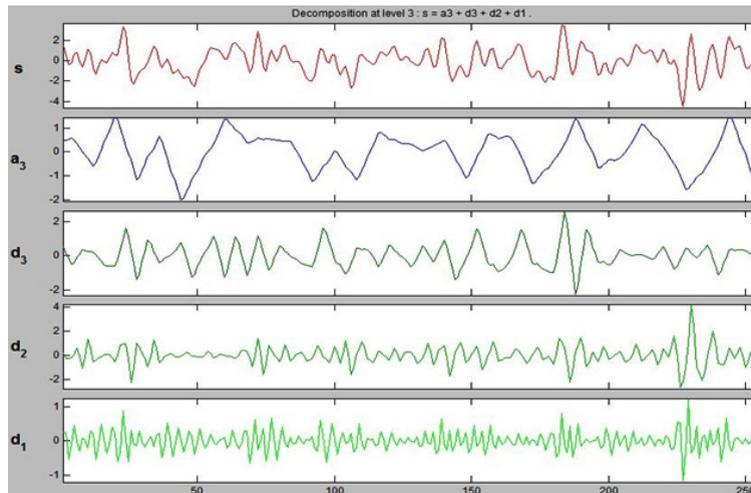
**Fig. 2.** Three Level wavelet decomposition of the EMG signal
