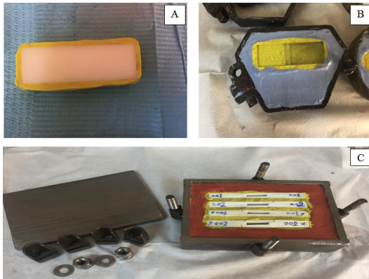
Fig. 2. A, The plastic pattern in silicone mold; B, Mold preparation for shear bond strength test; C, Custom fabricated flask with silicone –stone mold for final specimens
