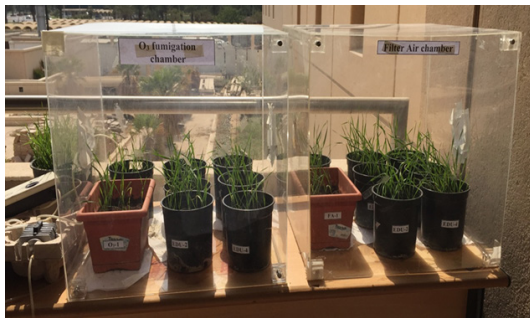
Fig. 1. Fumigation chambers: (a) Filter Air (FA) chamber. (b) Ozone
