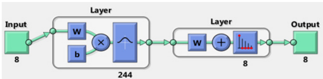
Fig. 6: Schematic of PNN network designed in Matlab
